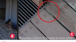
A Embers that pass through deck board gaps will land on the ground, or on combustible materials stored under the deck, as shown during this IBHS test.
