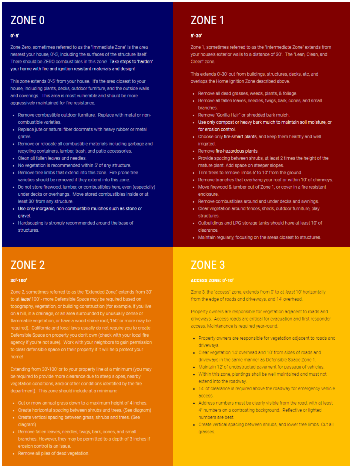
Figure 31. Description of the zones that make up the 100 feet of defensible space required by law ( https://www.firesafemarin.org/defensible-space ).
