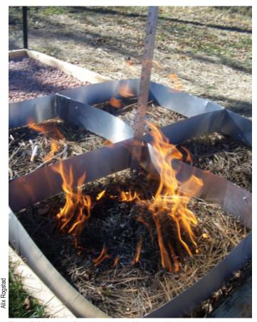
Figure 3. Measuring flame length in the 1/4 meter cell with a metal ruler.
