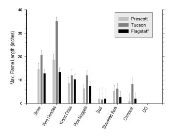
Figure 4. Average maximum flame length comparisons for each of the materials tested by study site with propane torch as ignition source. Bars represent mean flame length  $\pm$  standard error of the mean.
