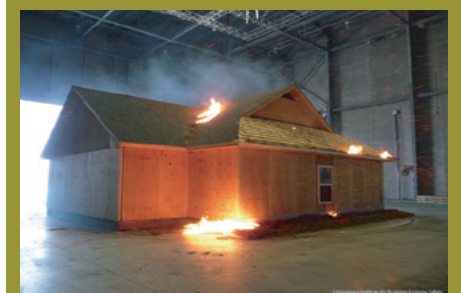
Photo 2. In order to be effective, external sprinklers must be able to wet all areas where ignition can occur, or be sufficiently effective in quenching embers that approach the home so they won't have enough energy to ignite combustible items.
