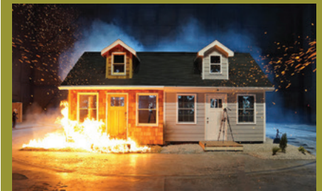
Figure 2b Embers impacting a building: left side with combustible (wood) and the right side with noncombustible (rock) mulch.
