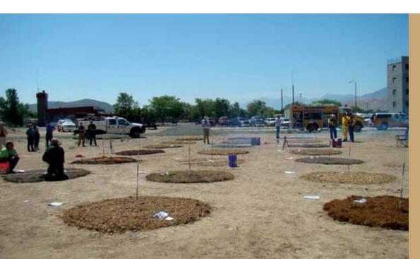
eight different mulch treatments were replicated three times and randomly positioned within the plot layout on May 28, 2008. After being exposed to the elements for over 2½ months, they were ignited on Aug. 14, 2008.
