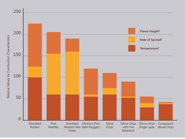
▲ Figure 3. Relative values of three combustion characteristics between eight mulch treatments. ¹Average maximum flame height. ²Average rate of fire spread. ³Average maximum temperature measured at four inches above the bed.
