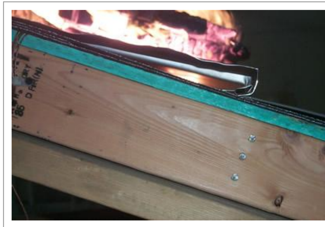
This aluminum roof covering is an assembly-rated Class A. The underlying Type 72 capsheet (roll roofing) material provides additional protections, and is required for the Class A rating.
